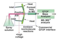
A blow-by-blow account: Extractive electrospray ionization (EESI) quadrupole TOF (QTOF) mass spectrometry has been established with a commercial instrument without hardware modification for the rapid analysis of breath without sample pretreatment (see picture). Sulfur-containing compounds can be selectively detected by using silver cationization in the EESI source—a method of interest for in vivo metabolic studies and clinical diagnosis.
